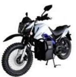
Motor Power :8000w Gears: Single Speed Battery:72V Lithium Battery Battery Capacity:>40Ah Range Per Charge: About 60km Max Speed:100km/h Net Weight(no battery):86kg Wheel Size:21" motorcycle tire Max load: 250kg
